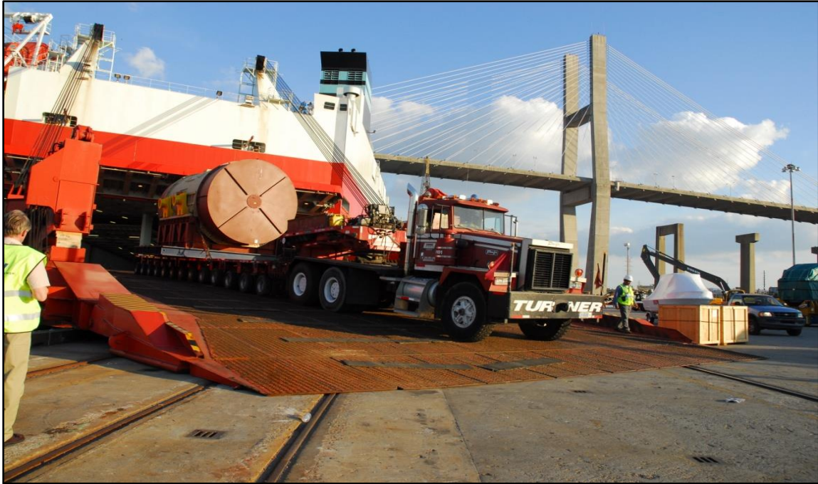
Equipment being off loaded on a "RO-RO" ship at Ocean Terminal
